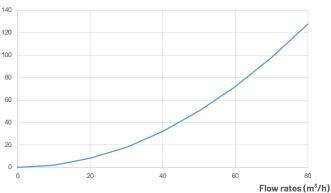
$^2$  Typical initial pressure drop  $\Delta P$  per 40" element, water at 20°C, viscosity
