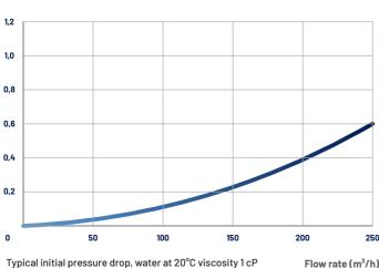
Typical initial pressure drop, water at 20°C viscosity 1 cP
