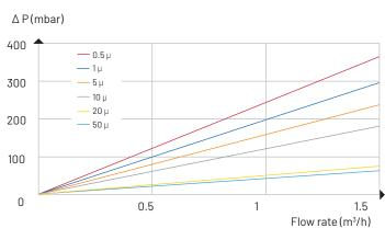
Typical initial pressure drop  $\Delta P$  per 254mm (10") element, water at 20°C, viscosity 1cP.
