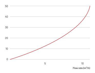
Typical initial pressure drop  $\Delta P$  per 254mm (10») element, water at 20°C, viscosity 1cP.
