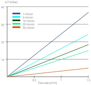
Typical initial pressure drop per 254mm (10") element, water at 20°C, viscosity
