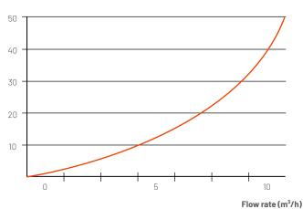
Typical initial pressure drop  $\Delta P$  per 10" element, water at 20°C, viscosity
