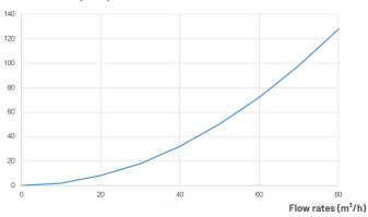
$^2$ Typical initial pressure drop  $\Delta P$  per 40" element, water at 20°C, viscosity 1cP
